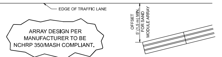
DETAIL "A" IMPACT ATTENUATOR, TEMPORARY (SEE NOTE 5)
