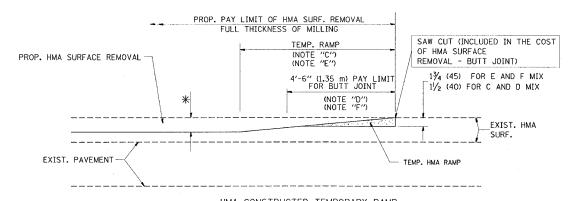
HMA CONSTRUCTED TEMPORARY RAMP
