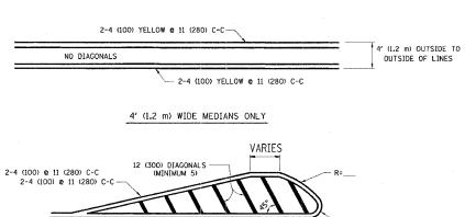
FOR MEDIAN LENGTHS WHERE DIAGONAL SPACING CANNOT BE ATTAINED, USE 5 (FIVE) EQUALLY SPACED DIAGONAL LINES.
