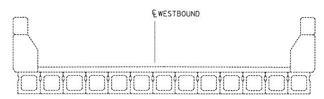
SUPERSTRUCTURE TO BE REPLACED REFER TO STRUCUTURAL PLANS FOR PROPOSED IMPROVEMENT
