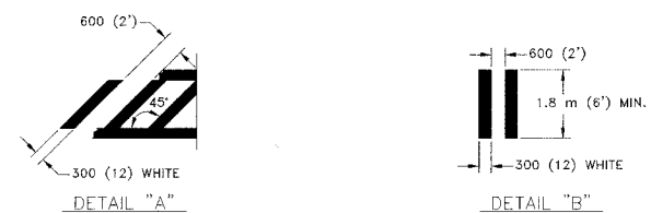
TYPICAL CROSSWALK MARKING
