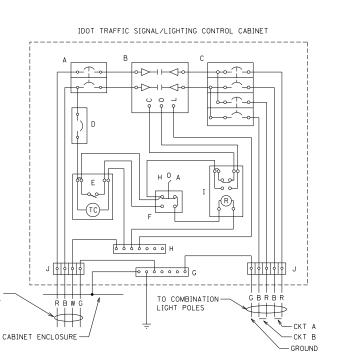
COMBINATION LIGHTING CONTROLLER WIRING DIAGRAM (NOT TO SCALE)
