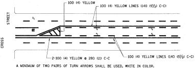
ADDITIONAL PAIRS SHALL BE PLACED AT 60 m (200') TO 90 m (300') INTERVALS.
