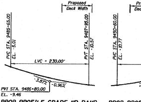
PROP PROFILE GRADE NB RAMP Alona @ NB RAMP
