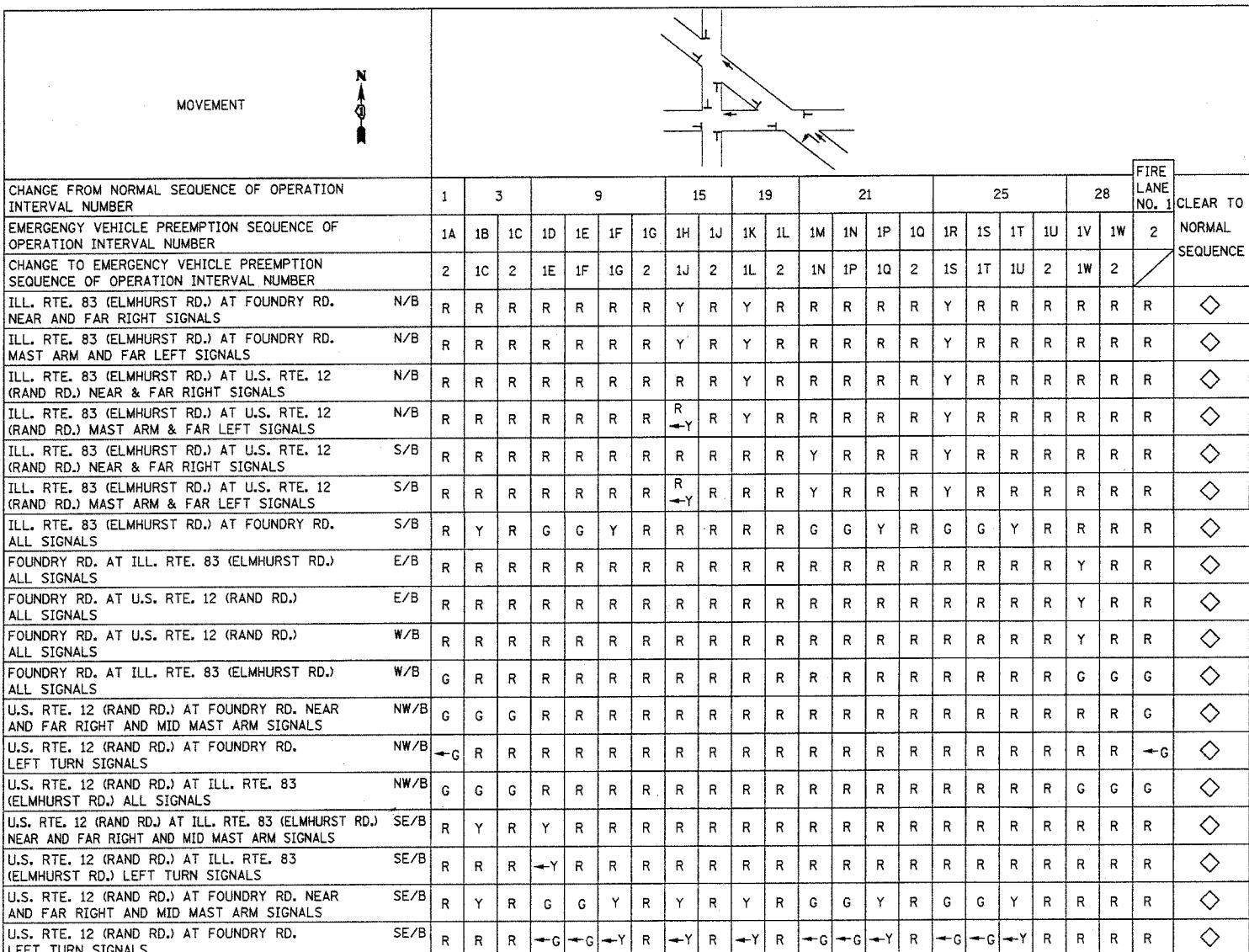
◆ EMERGENCY VEHICLE SEQUENCE SHALL PROVIDE THE PROPER CLEARANCE INTERVAL TO RESUME THE NORMAL SEQUENCE OF OPERATION OR PROPER CLEARANCE INTERVAL TO DISPLAY A DIFFERENT EMERGENCY VEHICLE INTERVAL AFTER EMERGENCY VEHICLE INTERVAL 2 OR 3 IS TERMINATED.
