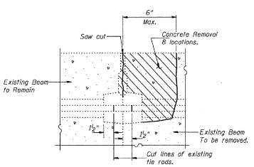
BEAM REMOVAL DETAIL AT TRANSVERSE TIES
