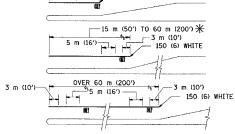
\* TURN LANES IN EXCESS OF 120 m (400') IN LENGTH MAY HAVE AN ADDITIONAL SET OF ARROW - "ONLY" INSTALLED MIDWAY BETWEEN THE OTHER TWO SETS OF ARROW - "ONLY".
