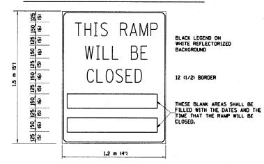
THESE SIGNS ARE REQUIRED ON BOTH SIDES OF THE RAMP, 4 MINIMUM OF 1 WEEK IN ADVANCE OF THE CLOSURE.
