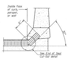
AT CURB, PARAPET, OR WALL (Showing seal)
