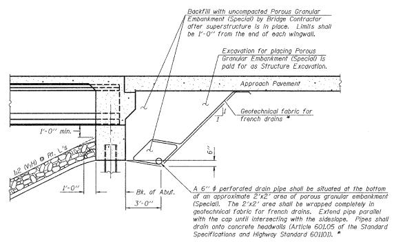
\* Included in the cost of Porous Granular Embankment (Special).
