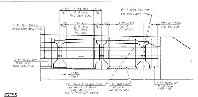
DIAPHRAGM ELEVATION AT ABUTMENT
