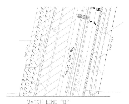
NOTE: THE VIDEO DETECTION ZONES SHOWN ON THE PLANS ARE FOR PRE-CONSTRUCTION STAGE (EXISTING GEOMETRICS) AND SHALL BE REDEFINED FOR EACH CONSTRUCTION STAGE AS A PART OF "TEMPORARY TRAFFIC SIGNAL INSTALLATION" WORK.
