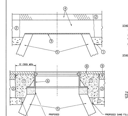
BRICK, MORTAR, OR CONC. ADJUSTING RINGS
