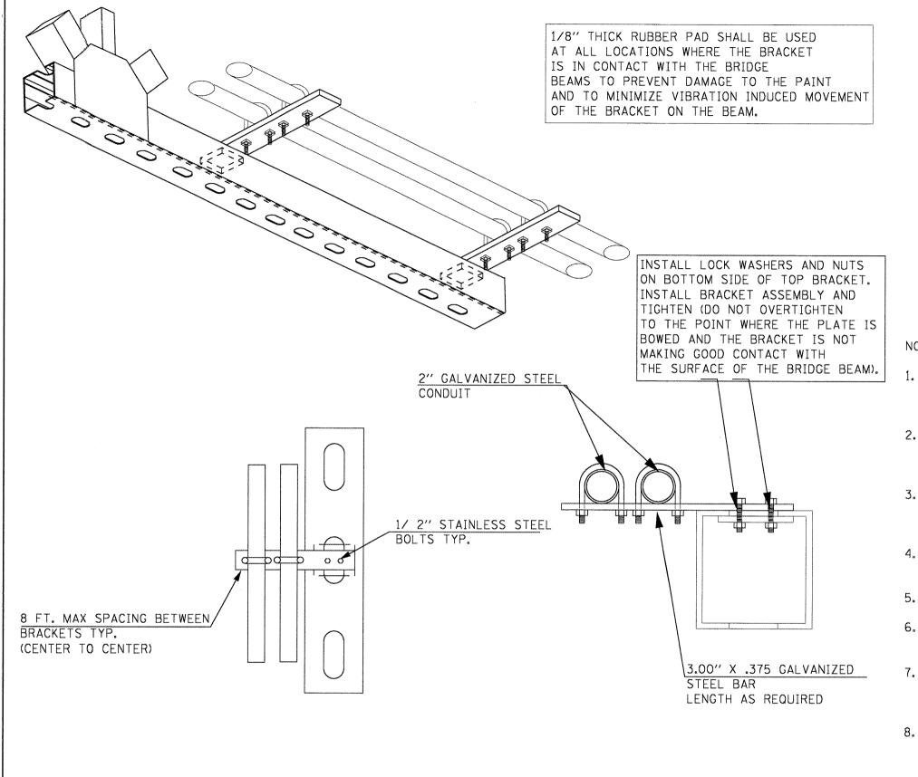
CONDUIT ATTACHMENT ON SUPERSTRUCTURE BOX BEAM
