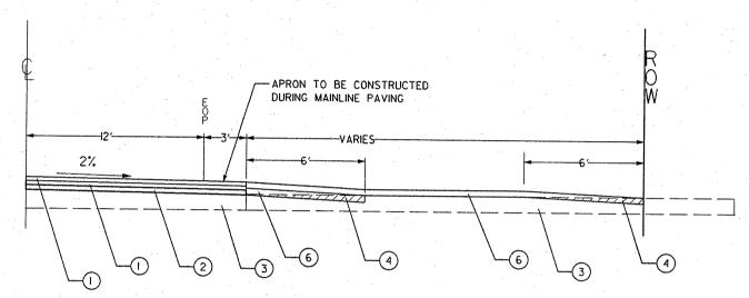
ENTRANCE NO.13 TO BE SAWCUT WITH BUTT-JOINT AT ROW LIMITS.
