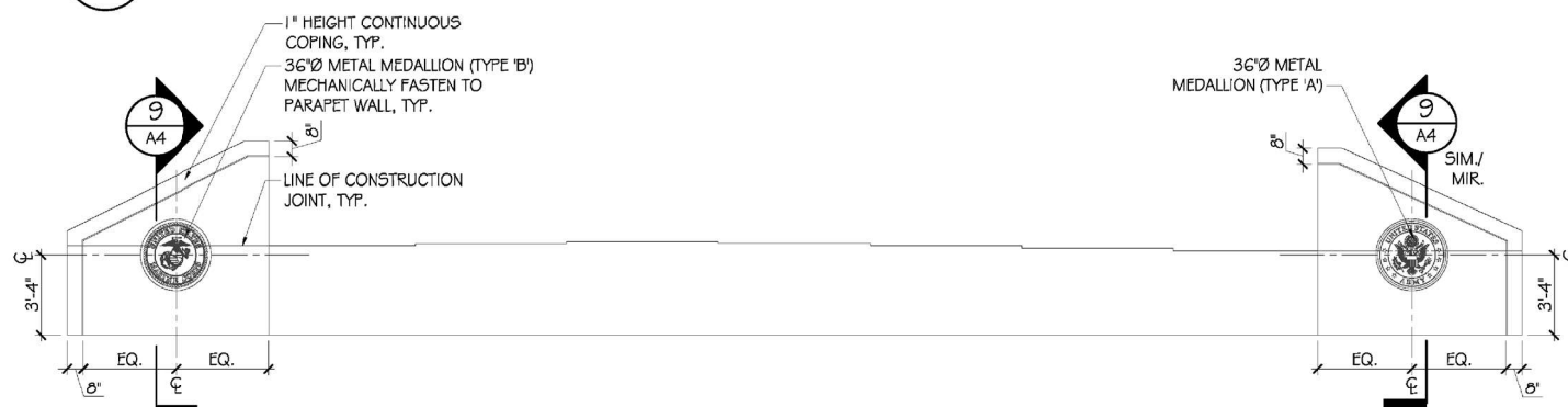
3 EAST ABUTMENT ELEV: WEST FACE A3 SCALE: 1/4" = 1'-0"
