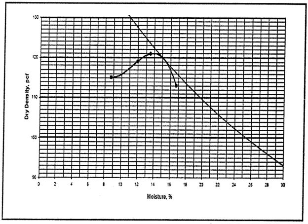
Zero Air Void Curve Specific Gravity: 270
