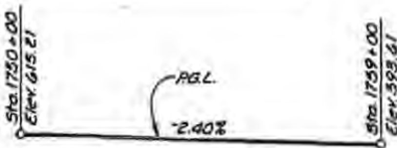
FAI 74 PROFILE GRADE (Along E Pavement)
