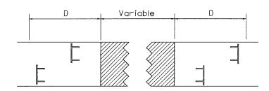
Type III Barricades and R11-4-4830 signs shall be as shown in "Road Closed To All Thru Traffic" detail on Highway Standard 702001. If the distance "D" exceeds 600 m (2000") an additional set of barricades and R11-4-4830 shall be placed at each end of the work area.
