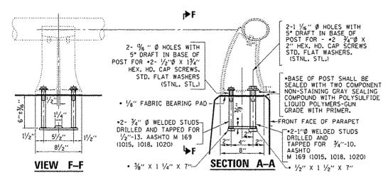
• NEW RAIL POST ANCHORAGE DEVICES WILL BE REQUIRED AT EACH LOCATION WHERE POSTS ARE CONNECTED TO NEW CONSTRUCTION. COST SHALL BE INCLUDED WITH REMOVING AND RE-ERECTING EXISTING RAILING.
