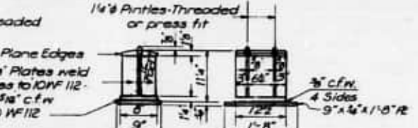
DETAIL OF BEARING AT ABUT. 1
