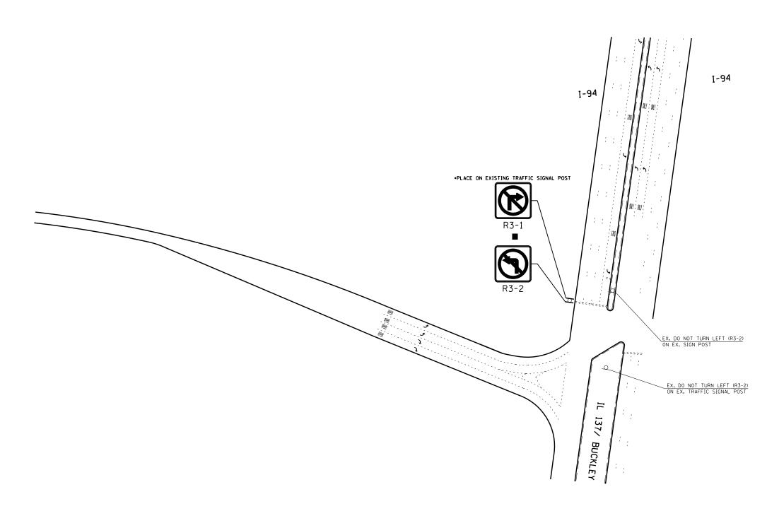
NOTE: SIGN ASSEMBLIES GREATER THAN 16 SOUARE FEET REQUIRE 2 TELESCOPING STEEL SIGN SUPPORTS.
