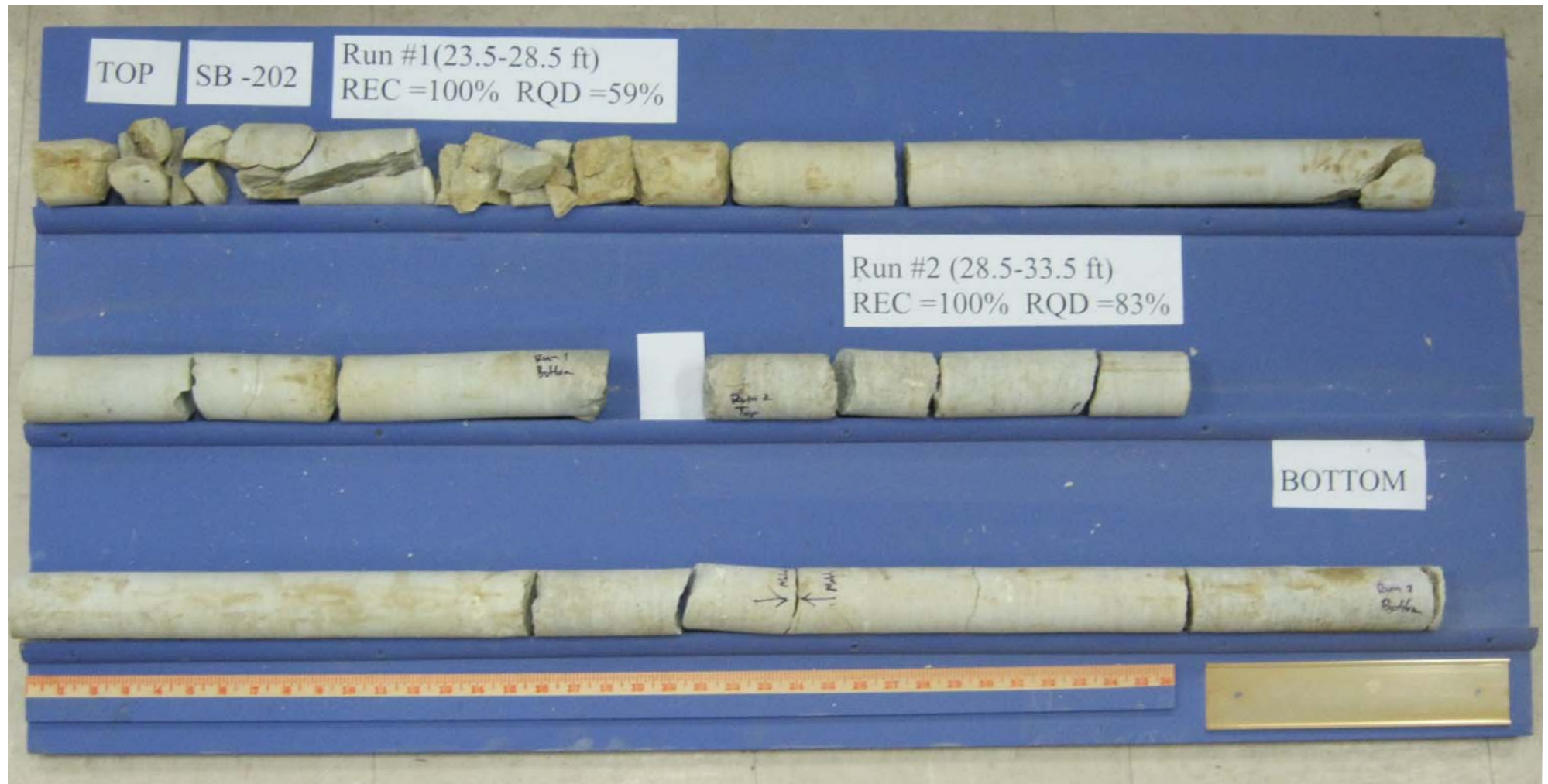
Boring SB-02: Run #1, 23.5' to 28.5', RECOVERY=100%, RQD=5% Run #2, 28.5' to 33.5', RECOVERY=100%, RQD=83%
