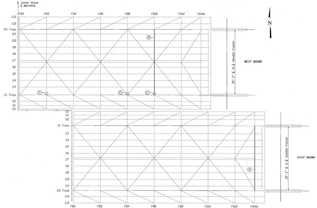
(B) Remove and replace floor beam lower flange angles
