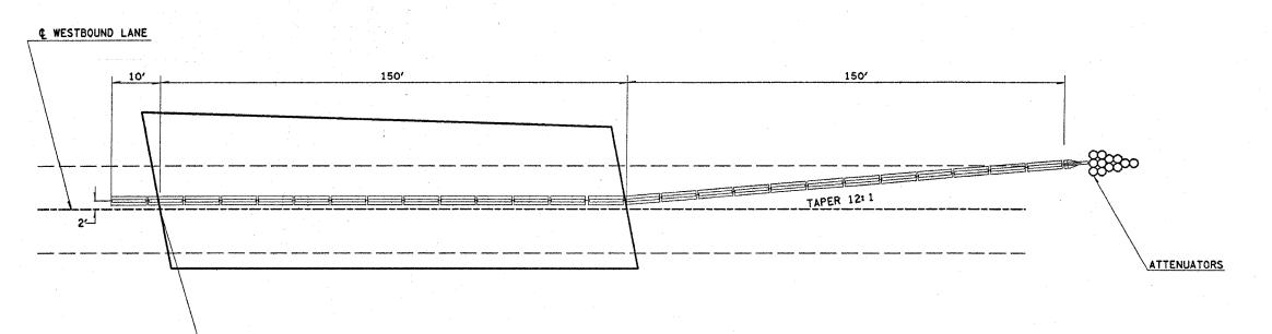
TEMPORAY CONCRETE BARRIER PLACEMENT DETAIL
