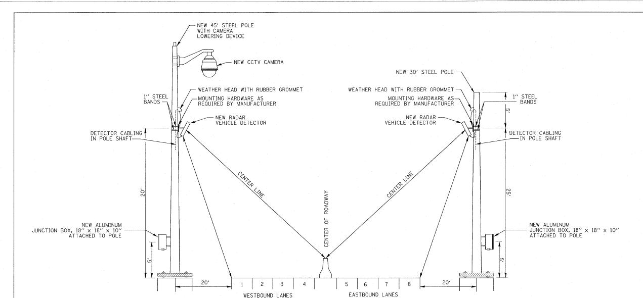
DETAIL RADAR VEHICLE DETECTOR NOT TO SCALE
