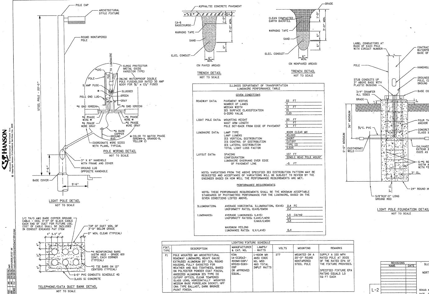
RTE. SECTION COUNTY 05-00001-01-PV DEKALB 38 19 TO STA. STA. C# 87319 ILLINOIS FED. AID PROJECT CONTRACTOR SHALL INSTALL BUSSMAN IN-LINE WATERPROOF FUSE HOLDERS WITH FUSE AT BASE OF POLE TO PROTECT FIXTURE WIRING. ~HANDHOLE WITH COVER GROUNDING LUG PROVIDED WITH POLE, CONNECT \*8 BARE GROUND WIRE TO ROD AND POLE -BASE COVER
