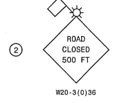
Post mounted sign with 18"  $\times$  18" (Minimum) orange flag and Type A Flashing Light.
