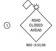
Post mounted sign with 18" x 18" (Minimum) orange flag and Type A Flashing Light.
