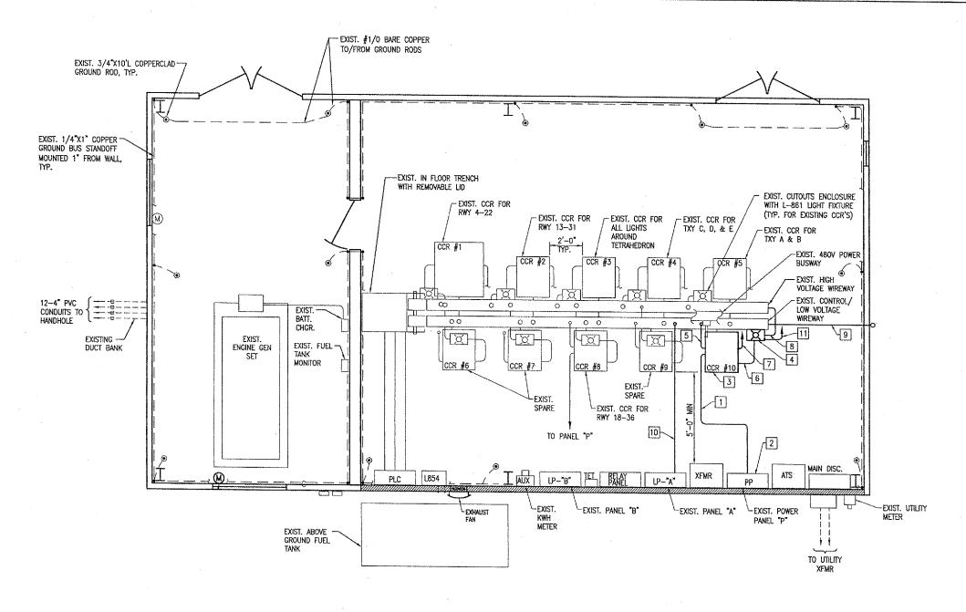
ELECTRICAL VAULT FLOOR PLAN
