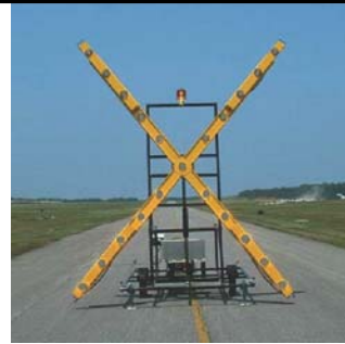
LIGHTED RUNWAY CLOSURE MARKER NOT TO SCALE
