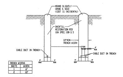
NOTE: TRENCH UTILIZING ADDITIONAL DUCTS SHALL BE WIDENED TO PROVIDE SPACING AS SHOWN.
