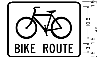
D11-1_24x18; 1.5" Radius, 0.5" Border, White on Green; Symbol RG025; [BIKE ROUTE] C 2K specified length;
