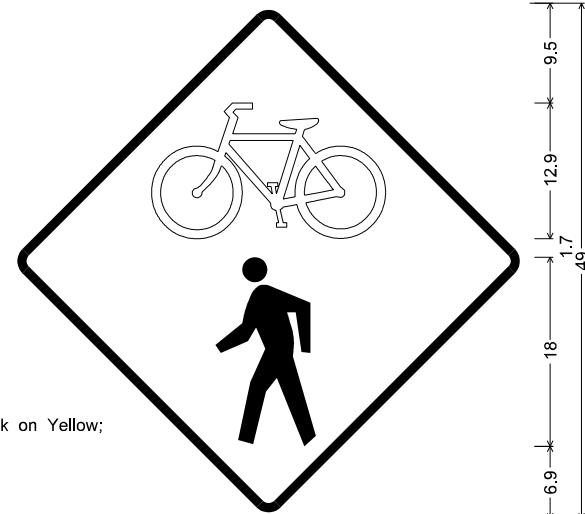
W11-15_36x36 FLYG; 36.0" across sides 2.3" Radius, 0.9" Border, 0.6" Indent, Black on Bright yellow green; Symbol RG025 Black;
