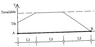
A = Front-end of reinforcement (at face of slope)
