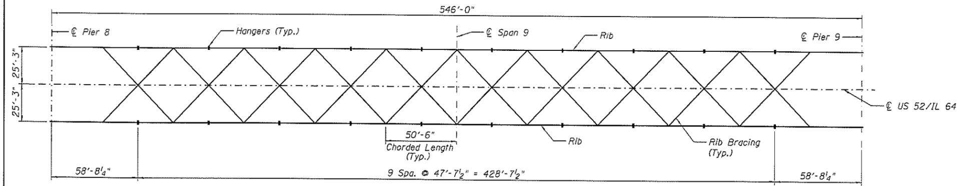
**RIB CROSS BRACING PLAN - UNIT 2**
