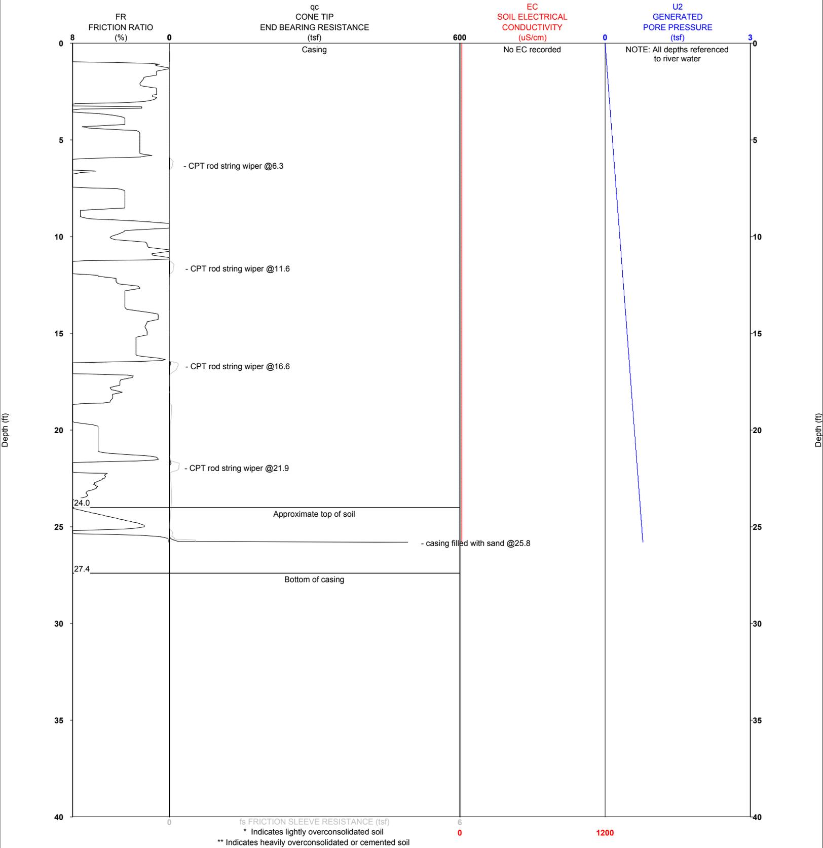
NOTE: Casing lowered and pushed into soil in inadvertent attempt to stabilize barge
