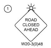
Post mounted sign with Type A Flashing Light
