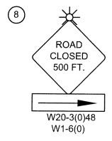
Post mounted sign with Type A Flashing Light
