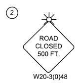
Post mounted sign with Type A Flashing Light
