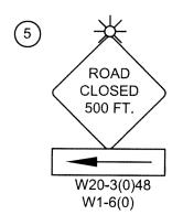
Post mounted sign with Type A Flashing Light
