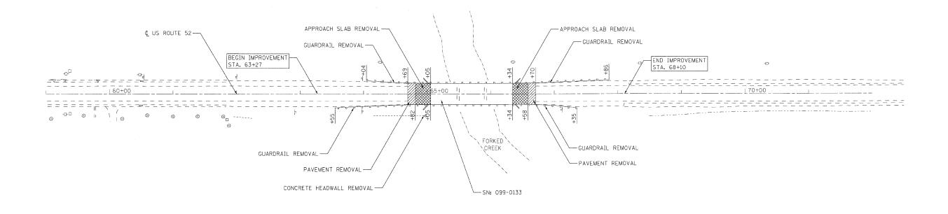
NOTE: THE EXISTING PAVEMENT CONSISTS OF 8 INCHES OF HOT-MIX ASPHALT OVER 9 INCHES OF PCC BASE COURSE.
