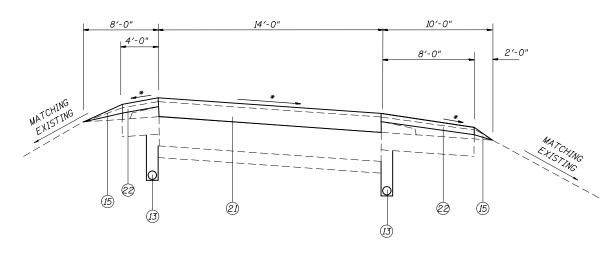
TYPICAL SUPERELEVATED RAMP SECTION
