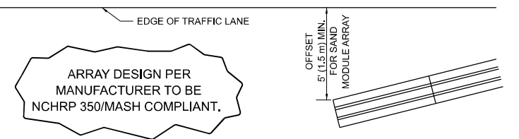
DETAIL "A" IMPACT ATTENUATOR, TEMPORARY (SEE NOTE 5)
