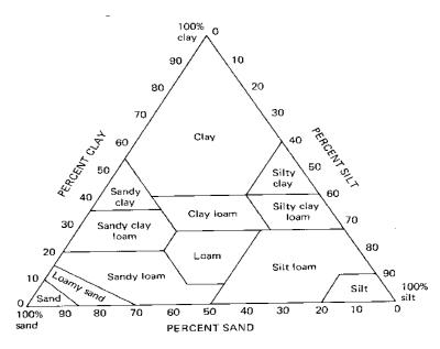
The mechanical analysis shall show that the % sand, % silt, and the % clay must yield a silt loam soil. See the attached Textural Classes diagram above. To determine the class plot a line parallel to the % clay axis starting the line at the value of the % silt. Plot another line parallel to the % sand axis starting the line at the value of the % clay. The intersection of these lines shall be in the silt loam region, for the soil to be approved.
