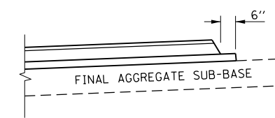
TEMPORARY PAVEMENT DETAIL - STAGE 1 (USE AT ALL TEMPORARY PAVEMENT LOCATIONS THIS STAGE)
