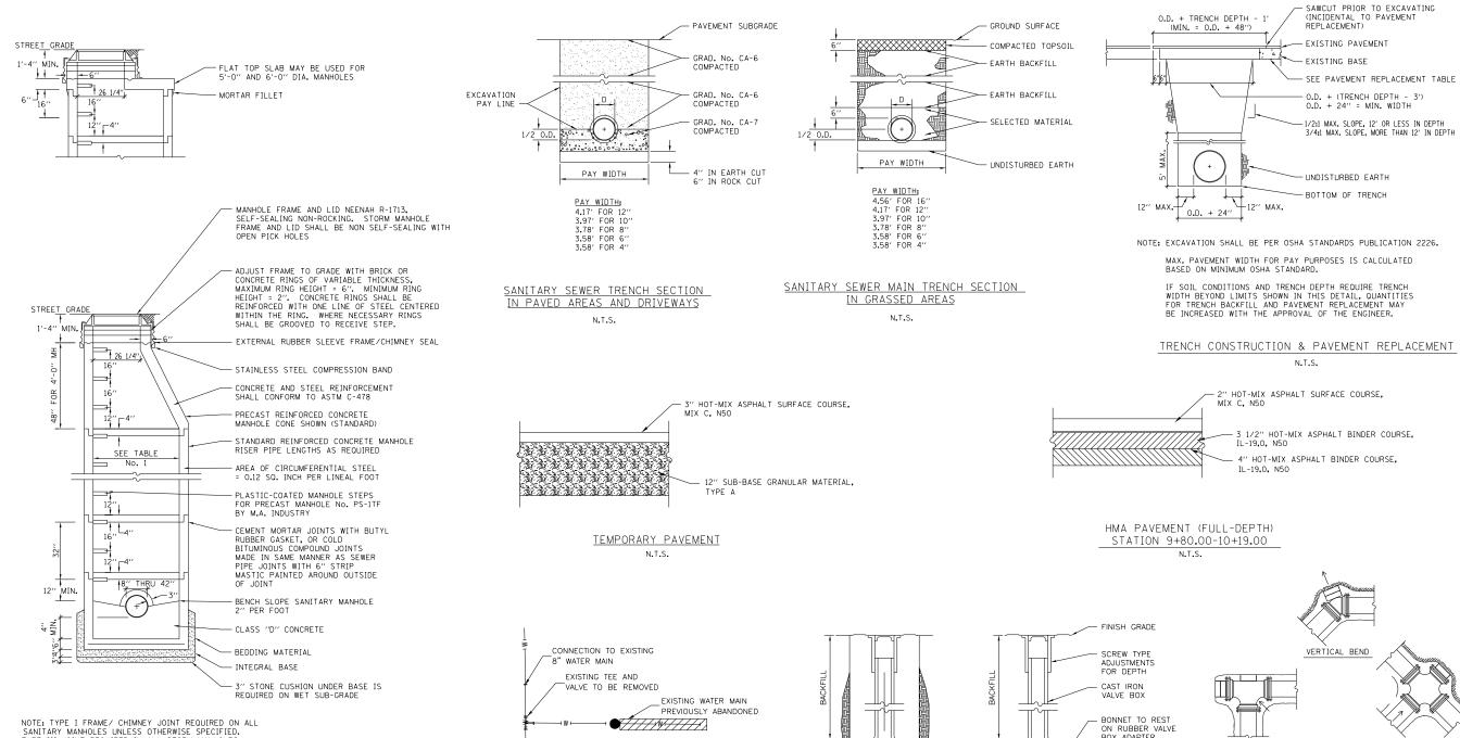
TYPE III JOINT REQUIRED IN ALL STORM MANHOLES
