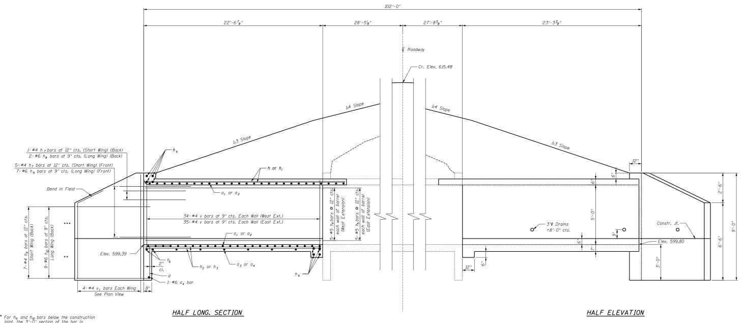
\*\* For h<sub>9</sub> and h<sub>10</sub> bars below the construction joint, the 3'-0" section of the bar is turned into the toe wall.
