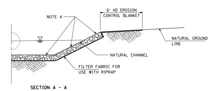
NOTE A - TRANSITION BASIN TO CONFORM TO THE NATURAL STREAM CHANNEL. TOP OF RIPRAP IN THE FLOOR OF THE BASIN SHOULD BE AT THE SAME ELEVATION OR LOWER THAN THE NATURAL CHANNEL BOTTOM AT SECTION " & SECTION ".
