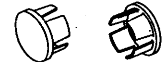
CAST END CAP DRIVE FIT TYPE 4 - Required Incidental to item "Aluminum Handrail"
