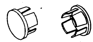
CAST END CAP DRIVE FIT TYPE 4 Required Galvanize to A.S.T.M. A-153. Incidental to item "Metal Handrail".
