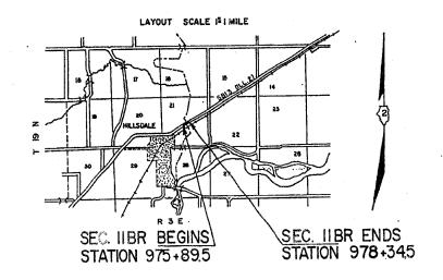
SECTION II BR INCLUDES THE REMOVAL OF THE EXISTING SUPERSTRUCTURE AND PORTIONS OF THE SUBSTRUCTURE AND REPLACEMENT WITH A PRECAST PRESTRESSED DECK BEAM BRIDGE OVER MEREDOSIA SLOUGH. ALSO INCLUDED IS CONSTRUCTION OF A TEMPORARY BRIDGE AND RUNAROUND AND ALL OTHER WORK THAT IS NECESSARY TO COMPLETE THE SECTION.
