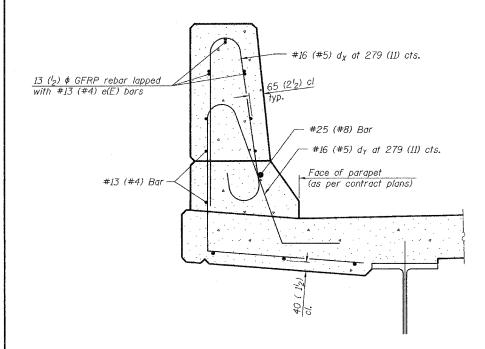
SECTION (Showing required reinforcement)
